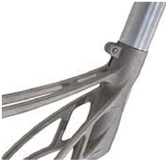
Figure 5 Empire Cycles, Seat adjustment detail 2014, 3D printed titanium frame with traditional seat post.
