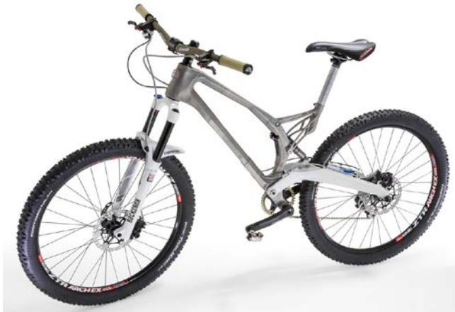
Figure 1 Empire Cycles, 3D printed bicycle frame 2014, 3D printed titanium frame with standard bicycle components attached.
