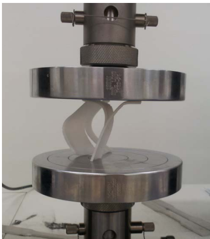
Figure 18 James Novak, Compression of a Tube – Horizontal 2014, ABS plastic printed on an 'Up! Plus 2' printer.
