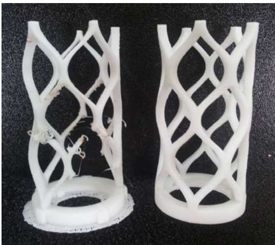
Figure 12 James Novak, Comparison of 3D printed lattice with different wall sections 2014, ABS plastic printed on an 'Up! Plus 2' FDM printer.
