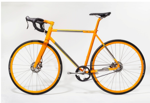
Figure 3 Flying Machine F-ONE-HD 2014, Frame constructed from 3D printed titanium lugs and extruded titanium tube with standard bicycle components attached.
