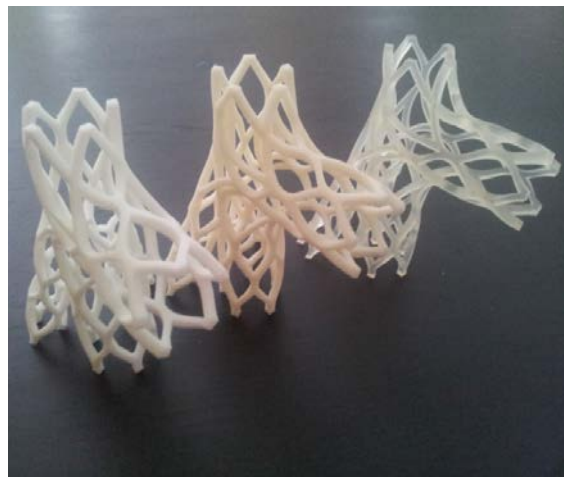
Figure 13 James Novak, Comparison of the same file printed on three different university printers 2014, left is ABS plastic from the 'Up! Plus 2,' middle is ABS plastic from the 'Fortus 250mc,' right is UV cured resin from the 'Projet HD 3500.'
