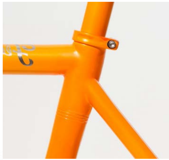
Figure 6 Flying Machine, Seat adjustment detail 2014, 3D printed titanium lug with traditional seat post.
