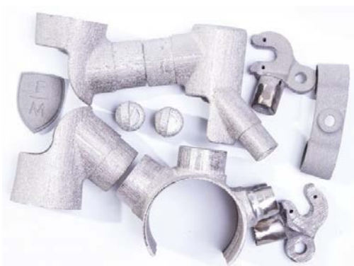
Figure 4 Flying Machine, 3D printed lugs 2014, 3D printed titanium.
